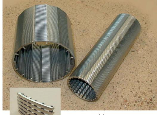
Wedge shaped wire construction welds stainless steel rods in precise alignment to achieve the best combination of flow rate and strength.
